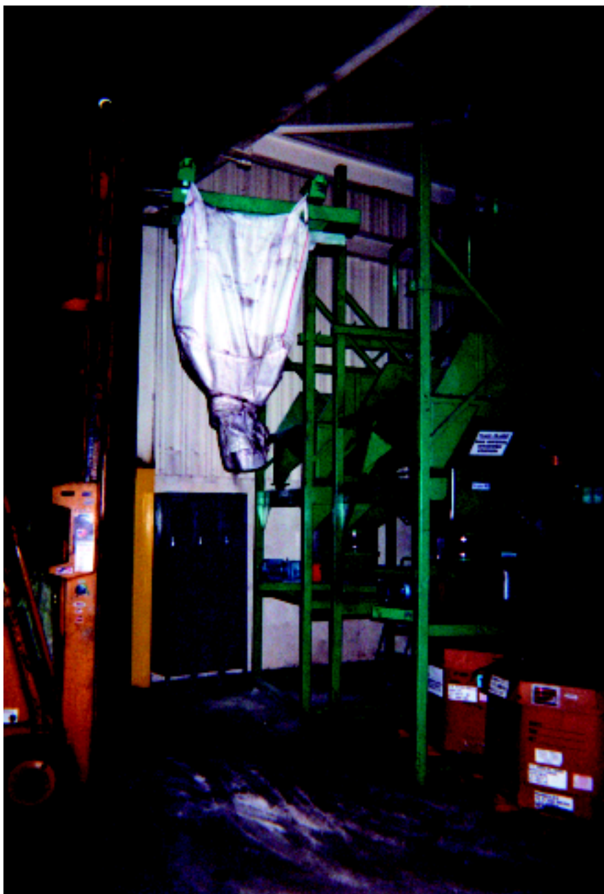
An operator uses a forklift to lift the bag-lifting frame and empty bag from the unloader.
