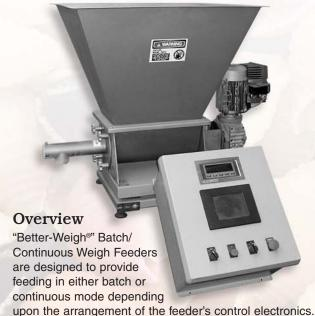
In batch mode, the batch controller is used to control the fast (bulk) and slow (dribble) speeds of the feeder. Accuracies of  $\pm 0.5\%$  can be easily achieved in 2 lb. or less batches, and  $\pm 0.25\%$  with 3 lb. or greater batches with time spans of 30 to 90 seconds. In continuous mode, the feeder's electronic controller is used to constantly monitor loss-of-weight of material per time in order to maintain a continuous loss-of-weight with an accuracy of  $\pm 0.25\%$  to 0.50%.
