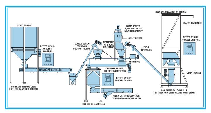
Sample artwork configuration showing the wide range of available Metalfab equipment that can be integrated into a complete dry solids material handling system or subsystem.
