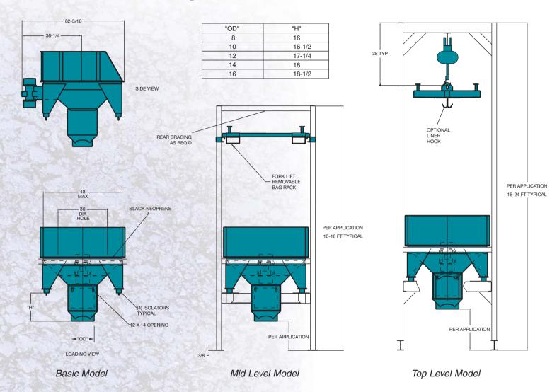
Contact Parts: Carbon steel, epoxy-coated carbon steel, 304 or 316 stainless steel External Structure: Carbon steel that is primed and painted blue enamel
