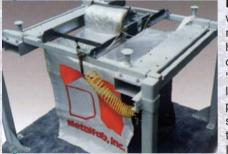
Bag Liners are easily handled with a pneumatically-powered, rubber covered pulley assembly held in bearings and fixed to the center of the bag rack with two "quick action" clamps. When the lined bag is placed into proper position for discharge, the bag is suspended from the bag rack while the liner is clamped to the pulley. In operation, the pulley's air
